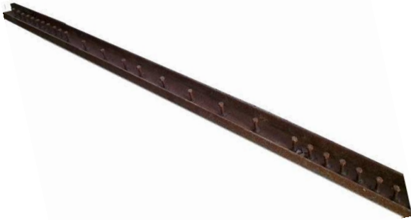
Plate 3: The steel channel with its attached headed studs for beam TB-NU45/90 .
