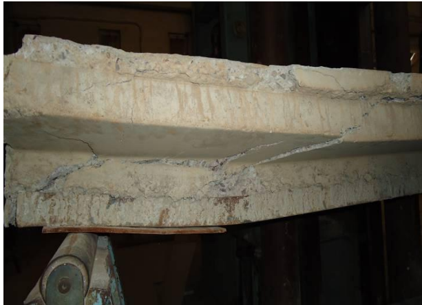
Plate 6: View of a typical tested beam after failure showing the fracture pattern
